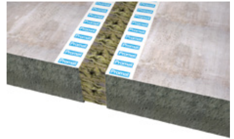
3. Compress mineral wool (melting point 1000 °C, class A1, density \geq 40 \text{ kg/m}^3 ) 30 % and insert in joint
